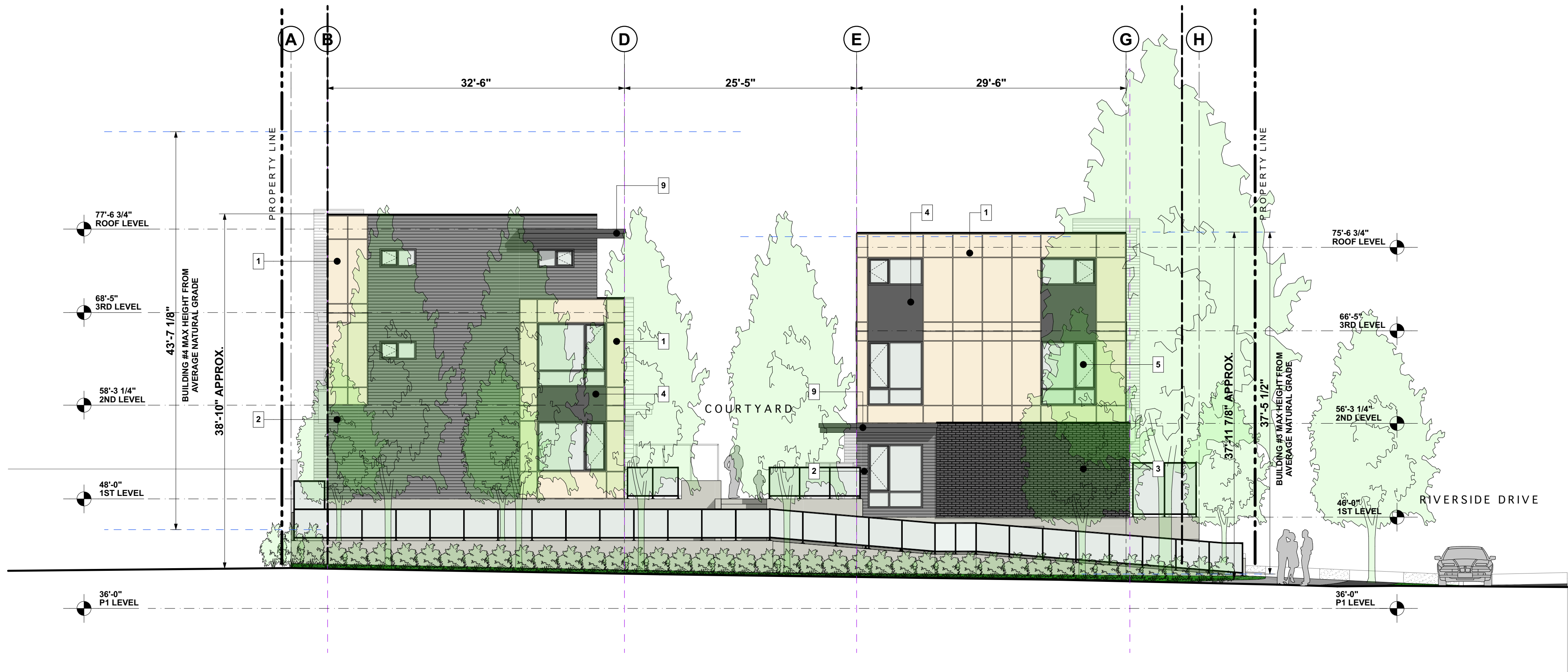
1 NORTH ELEVATION (MT. SEYMOUR PKWY) SCALE: 1/8" = 1'-0"
