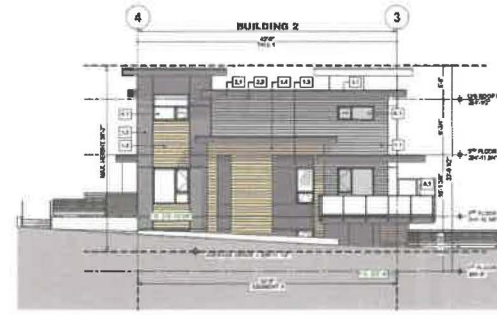
2 NORTH-WEST ELEVATION (NW) SCALE: 1/8" = 1'-0"
