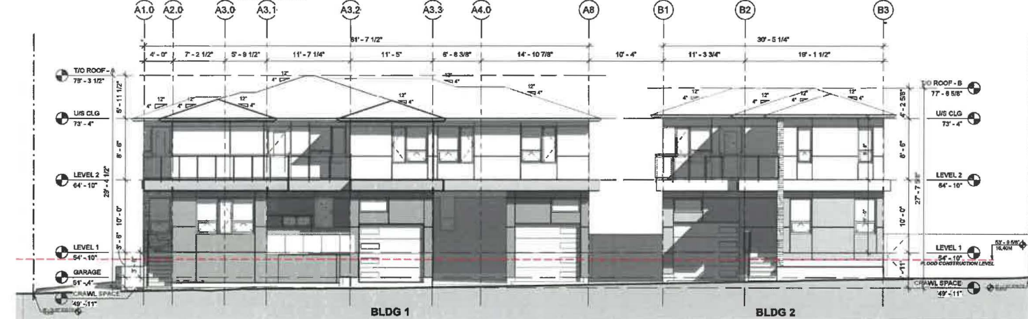
3-16 HT CALC SOUTH ELEVATIONS 1. LIMITING DISTANCE = 11.41 FT (3.48M) 2. TOTAL WALL AREA = 864 SF (80.20 SM) 3. ALLOWABLE OPENINGS (CBC 2015 TABLE 9.10.15.4) SPRINKLERED BUILDING = 20.85% X 2 = 41.7% = 357 SF 4. PROPOSED UNPROTECTED OPENINGS = 23 SF (2.14 SM) 5. CONSTRUCTION REQ'D (CBC 2015 TABLE 9.10.15.5) = 60 MIN. FRR COMBUSTIBLE OR NON-COMBUSTIBLE CONSTRUCTION & NON-COMBUSTIBLE CLADDING REQUIRED
