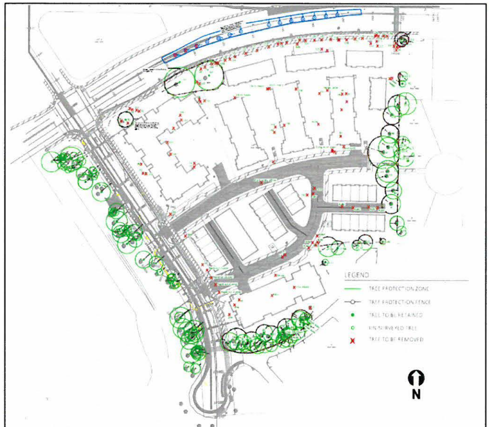
Figure 14. Tree Removal and Retention Plan
