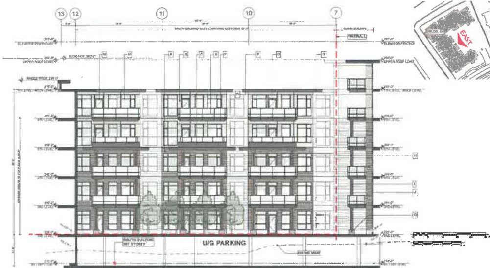
BUILDING 1 - EAST COURTYARD ELEVATION
