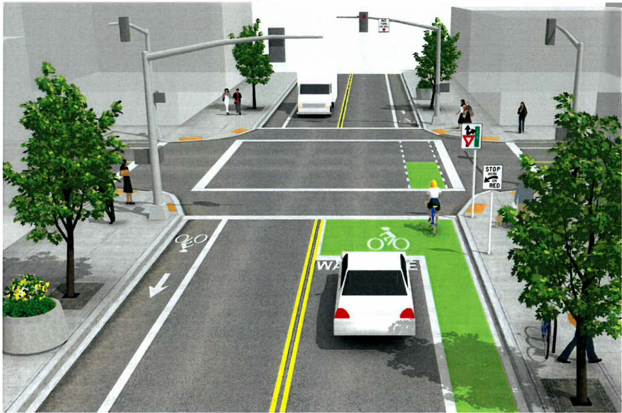
Figure 12. Typical Bike Box Treatment at Signalized Intersection (source: National Association of City Transportation Officials)
