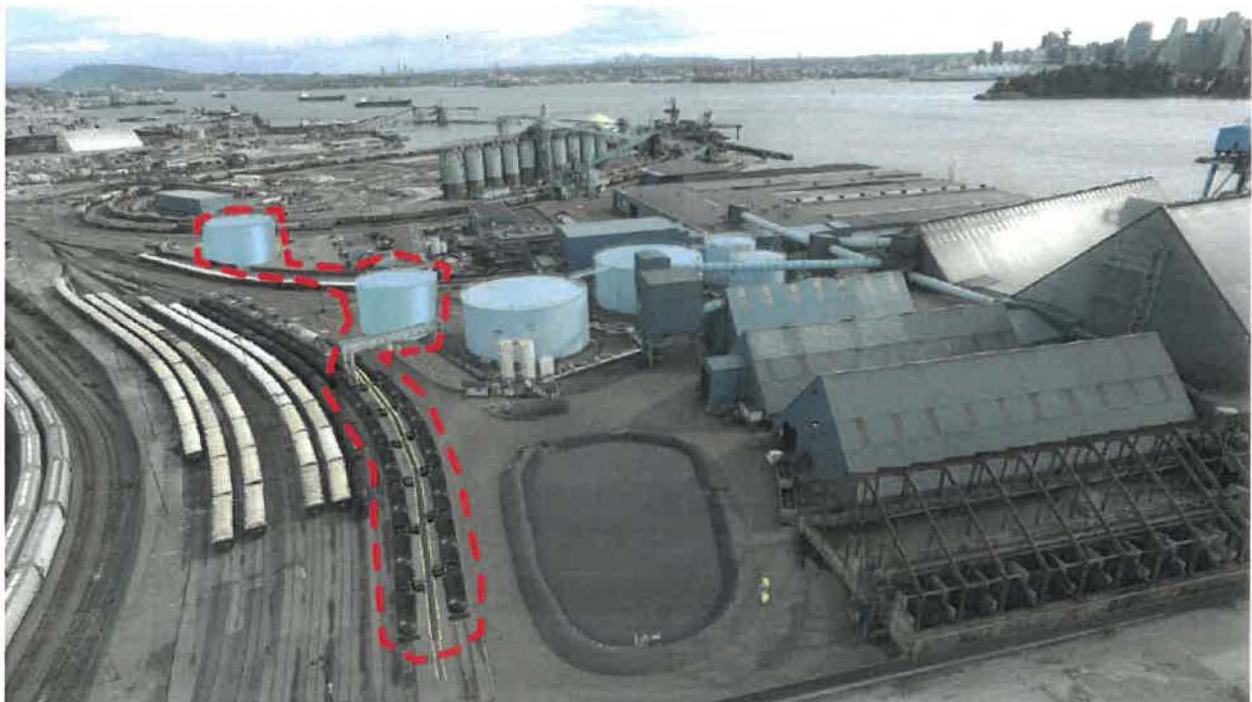
Rendering: Two new tanks and 12 new railcar unloading spots highlighted in red dashed line
