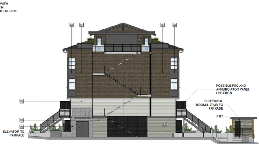
4 NORTH ELEVATION- BLDG 1 SOUTH SCALE: 1/8" = 1'-0"
