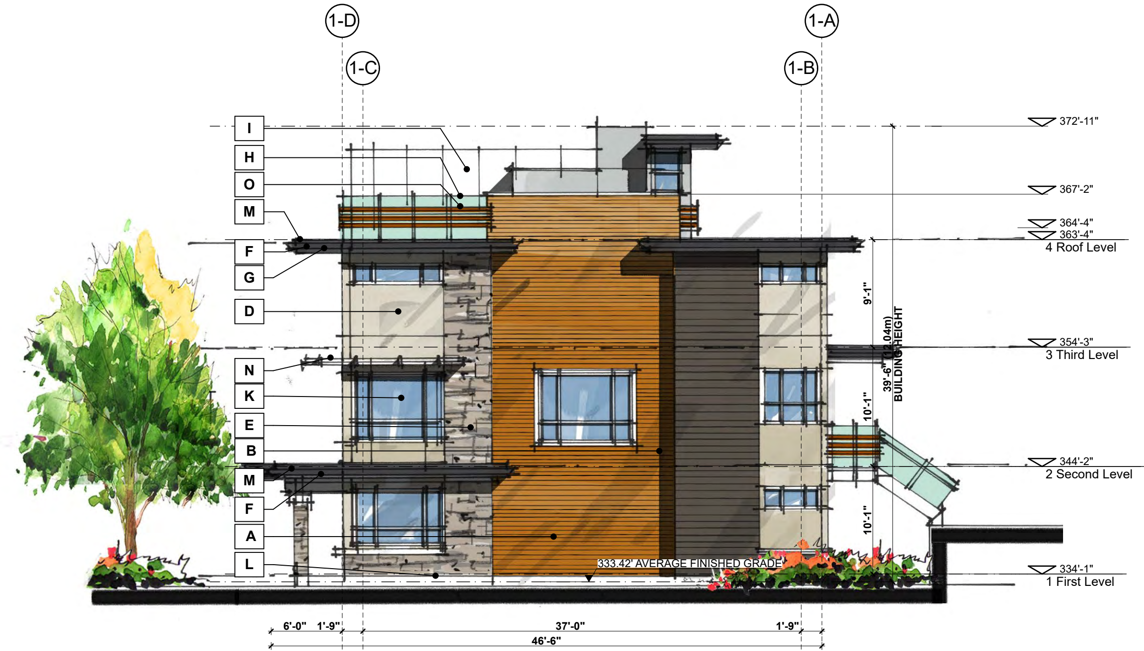
2 BUILDING 1 EAST ELEVATION SCALE: 1/8" = 1'-0"
