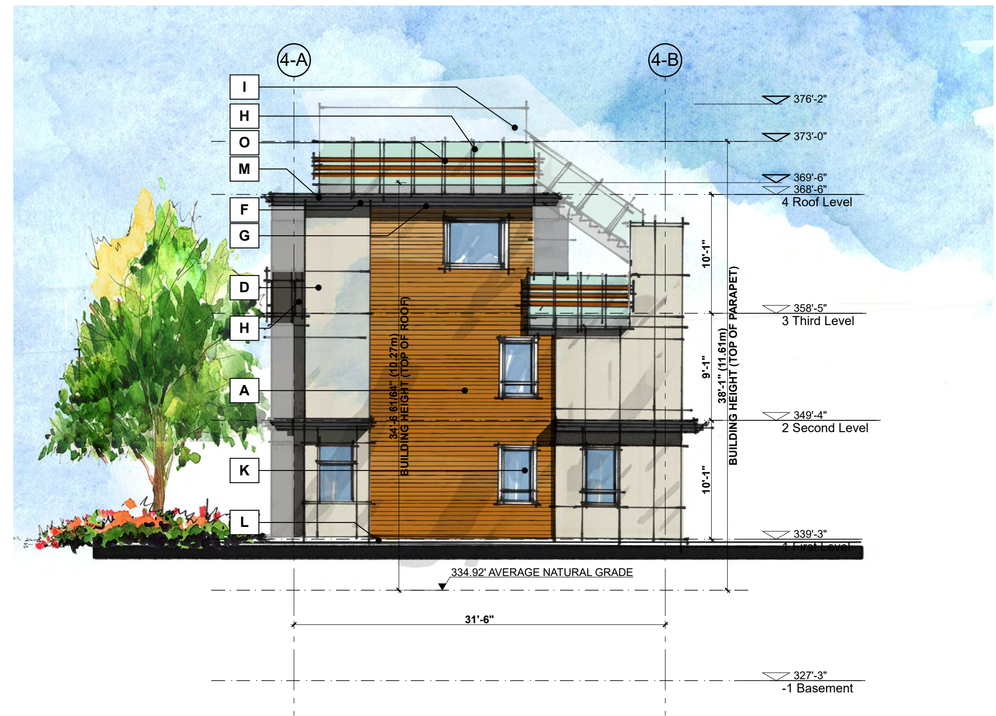
4 Building 4 West Elevation SCALE: 1/8" = 1'-0"
