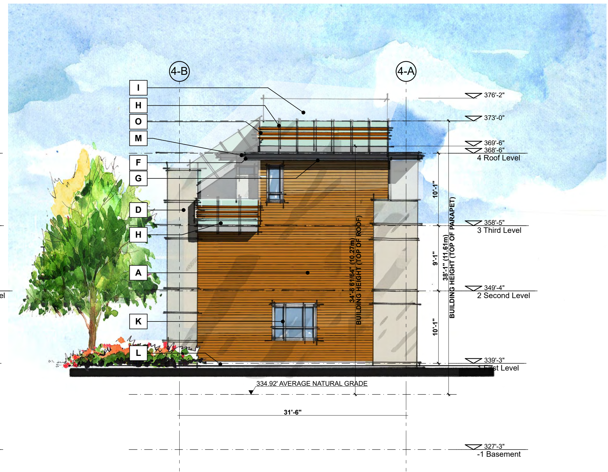
2 Building 4 East Elevation SCALE: 1/8" = 1'-0"
