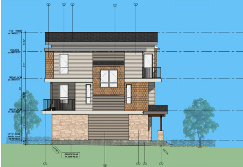
2 BUILDING 1 NORTH ELEVATION Scale: 3/16" = 1'-0"
