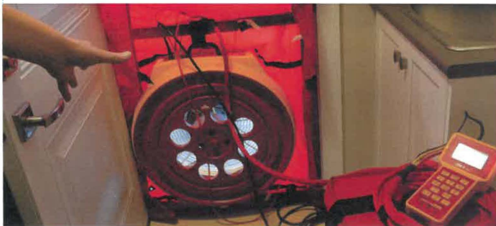
Figure 8: Blower door test in action
