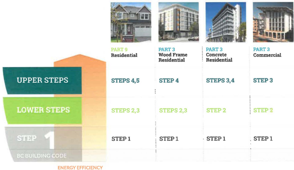
Figure 1: Definition of Lower and Upper Steps by building type (Part 9 and Part 3)
