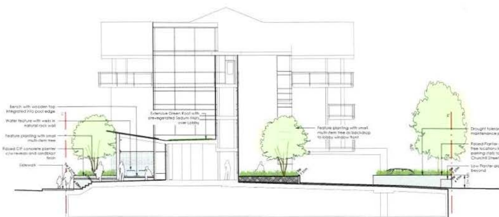
A Section-Elevation: Lobby Entry at Churchill Crescent, 2nd Level Common Patio and Drive Aisle at North Lane SCALE 1:100
