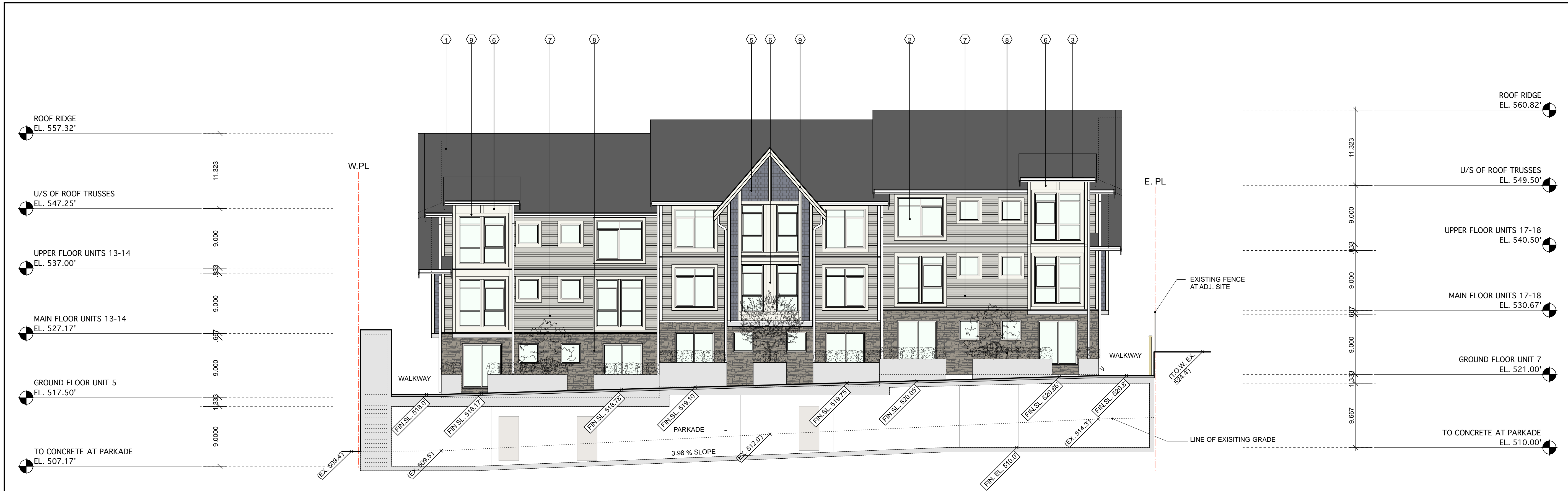
FRONT BUILDING - SOUTH ELEVATION (COURTYARD) SCALE: 1/8"=1'-0"
