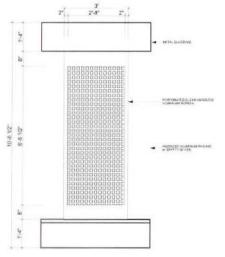
SCREEN SLIDER ELEVATION SCALE: 3/4" = 1'-0"
