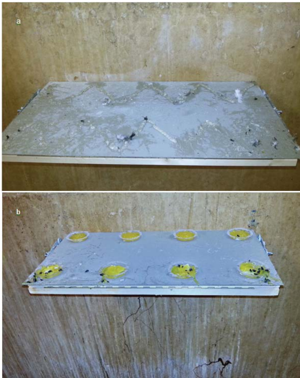
Figure 3. Appearance of the tactile gel (a) and the optical gel (b) after 23 days of application. Due to the adhesive effect numerous insects, feathers, dust and feces became stuck in the gels. The gluey optical gel got stuck on the wall underneath the experimental shelf when the pigeons stepped into the repellent and flew off pulling long adhesive strings. These remains were extremely difficult to remove.
