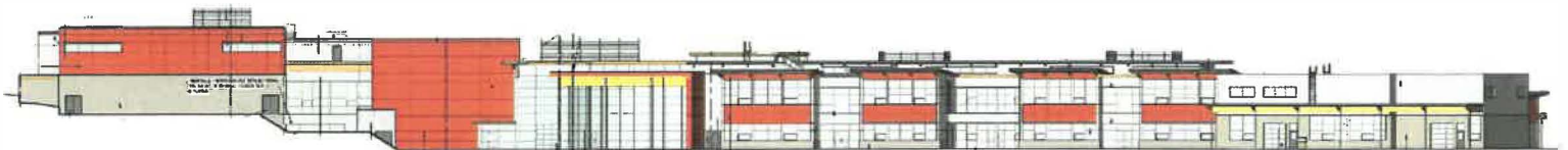
North elevation demonstrating how building conforms to the land profile of the site.
