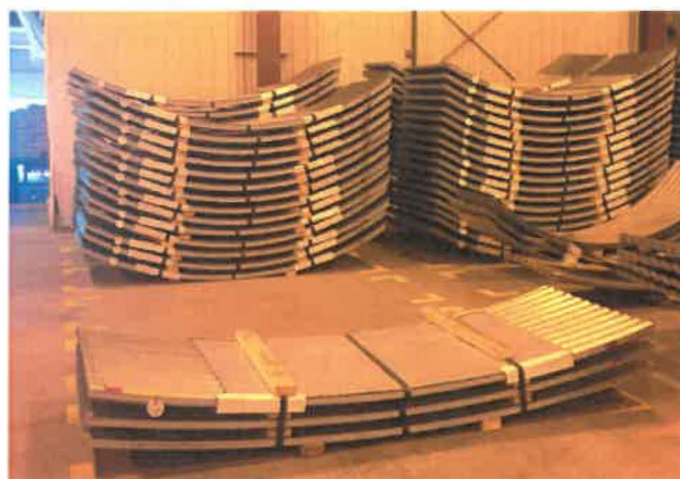
Silo wall components prior to delivery and assembly
