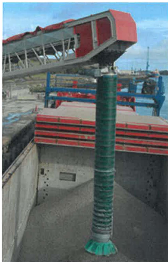
Example of telescoping unloading chute which mitigates dust
