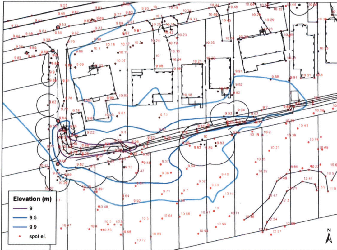
Figure 4: Elevation contours derived from the recent topographic survey showing potential inundation of floodwaters.
